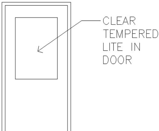
A "callout" is a leader line with text at its end. Leader lines are entered by using the LE command. Under this command there is a default variable that needs to be changed. This is changed in the "Triton D" template, but if you do not use the template and need to change it, type LE<RET><RET> Select the "Leader Line and Arrow" tab. Under the "Angle constraints" section, change the "Second segment" to "Horizontal." Click OK. <ESC>
