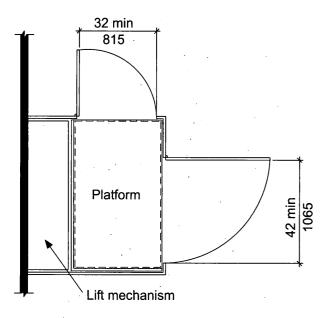
Fig. 410.2.1 Platform Lift Doors and Gates
