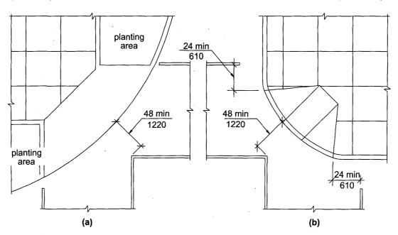
Fig. 406.10 Diagonal Curb Ramps
