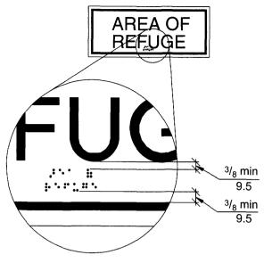
Fig. 703.4.4 Position of Braille
