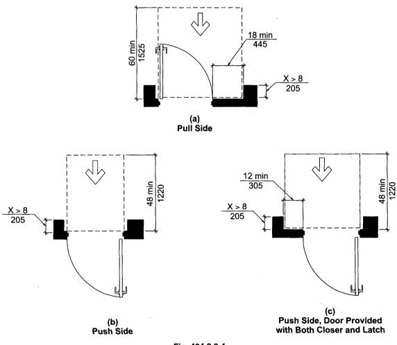
Fig. 404.2.3.4 Maneuvering Clearance at Recessed Doors
