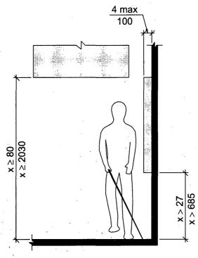
Fig. 307.2 Limits of Protruding Objects
