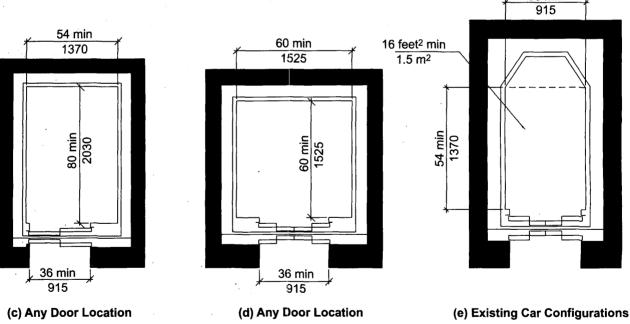
Fig. 407.4.1 Inside Dimensions of Elevator Cars
