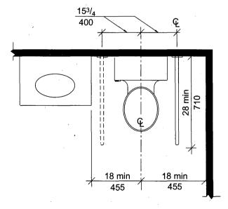
Fig. 604.5.3 Swing-up Grab Bar for Water Closet
