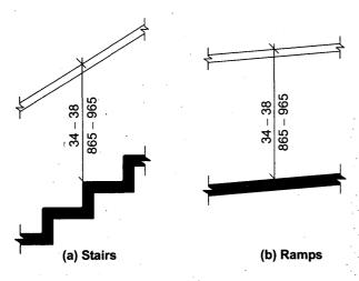
Fig. 505.4 Handrail Height
