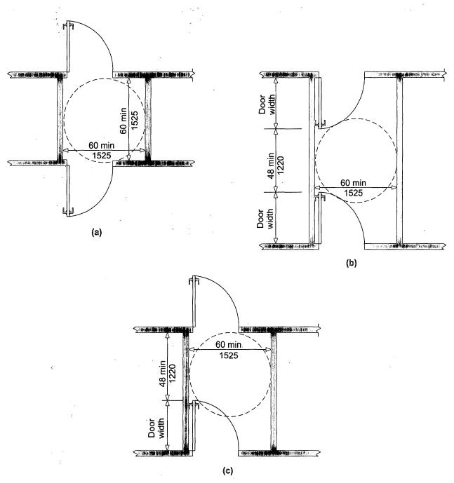
Fig. 404.2.5 Two Doors in a Series
