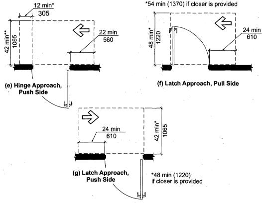
Fig. 404.2.3.1 **Maneuvering Clearance at Manual Swinging Doors**
