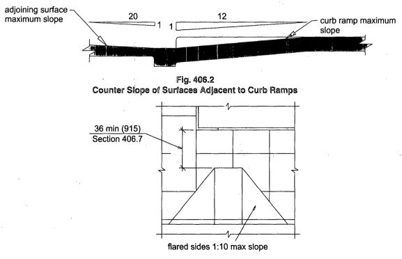
Fig. 406.3 Sides of Curb Ramps
