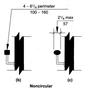
Fig. 505.7 Handrail Cross Section
