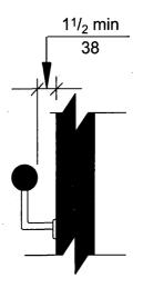
Fig. 505.5 Handrail Clearance
