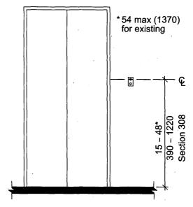
Fig. 407.2.1.1 Height of Elevator Call Buttons
