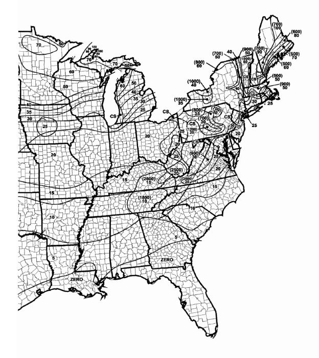
$$P_f = Snow | ord in psf = C_e \times C_t \times T \times P_g$$
